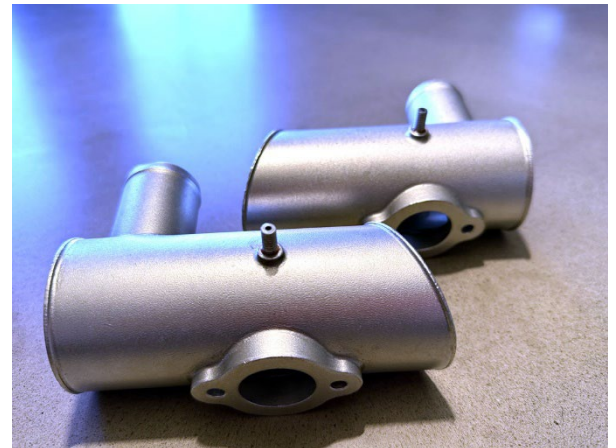
FIGURE 2. NOZZLE INSTALLED ON A STINGER PRO 125CC (STICKOUT IS LONG (>.200") AND WILL NEED TO BE CUT)
