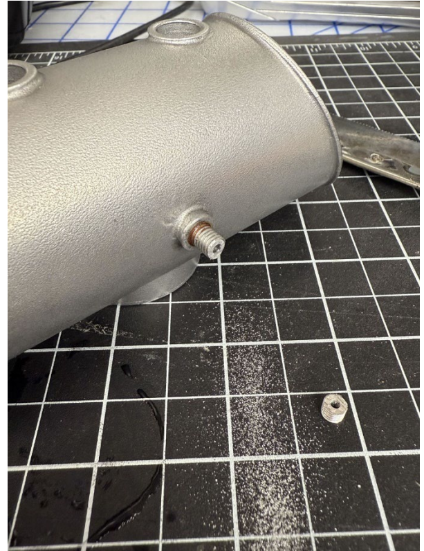
FIGURE 4. STICKOUT TRIMMED TO APPROX. 0.200" REINSTALLED AND LOCTITE APPLIED
