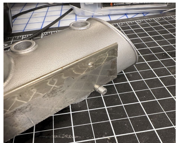
FIGURE 3. EXACTO SAW CUTTING THE NOZZLE TO LENGTH
